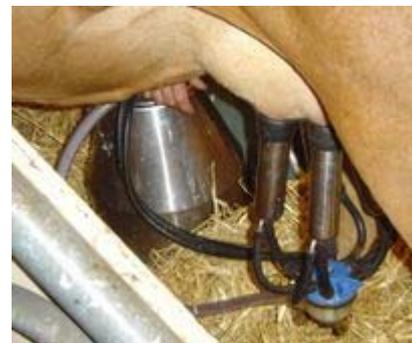
The four streams of milk from the teatcups are usually combined in the claw and transported to the milklime or collection bucket (usually sized to the output of one cow) in a single milk hose. Milk is then transported (manually in buckets) or with a mechanical pump to a central storage vat or bulk tank. Milk is refrigerated on the farm in most countries either by passing through a heat-exchanger or in the bulk tank.
